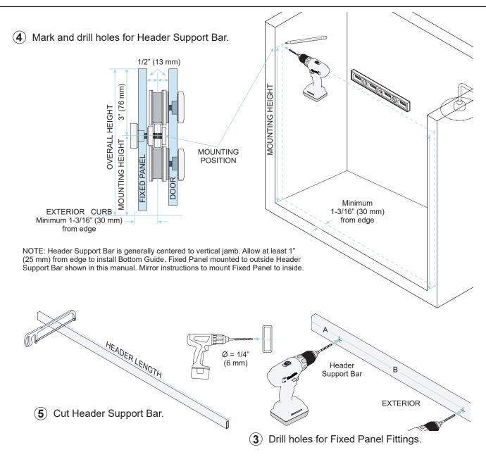
NOTE: Header Support Bar is cut 1" (25 mm) short from tight dimension and centered in opening, leaving 1/2" (13 mm) gap on each end to mount. Refer to Fixed Panel Glass fabrication and gap allowance between Fixed Panel and wall to determine mounting hole placement.
