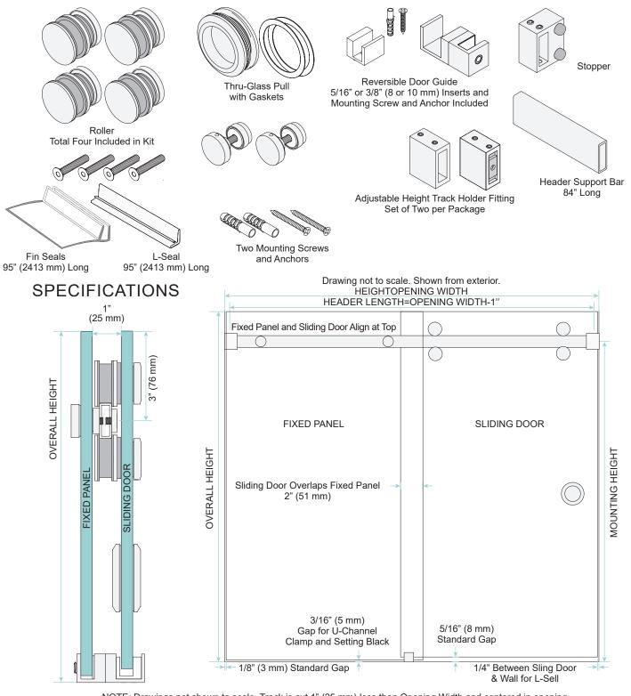
NOTE: Drawings not shown to scale. Track is cut 1" (25 mm) less than Opening Width and centered in opening. Overall Height is height from curb/floor to top of glass. Drawings shown from interior with Bottom Door Guide cupping Fixed panel.
