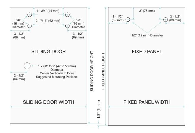
SLIDING DOOR AND FIXED PANEL WIDTH : Overall Width Divided by 2, plus 7/8" (22 mm) FIXED PANEL HEIGHT : Overall Height minus 3/16" (5 mm) SLIDING DOOR HEIGHT : Overall Height minus 5/16" (8 mm)
