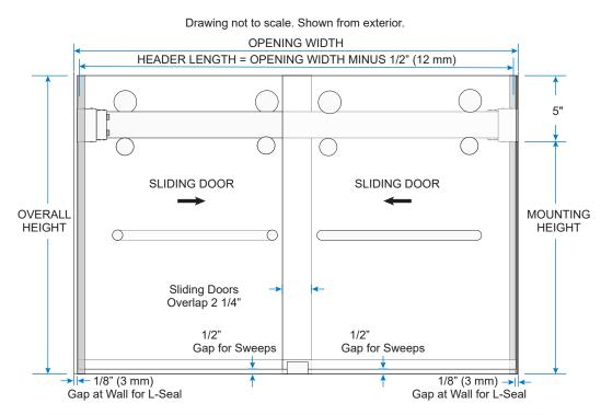
NOTE: Drawings not shown to scale. Header Bar is cut 1/2" (12 mm) less than Opening Width. Use wall-to-wall tight dimension.Overall Height is height from curb/floor to top of glass.
