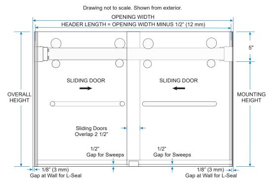
NOTE: Drawings not shown to scale. Header Bar is cut 1/2" (12 mm) less than Opening Width. Use wall-to-wall tight dimension.Overall Height is height from curb/floor to top of glass.
