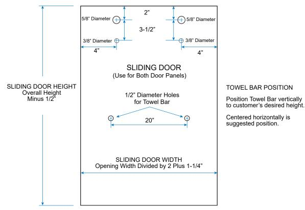
**SLIDING DOOR HEIGHT:** Overall Height minus 1/2" **SLIDING DOOR WIDTHS:** Overall Width divided by 2, plus 1-1/4"
